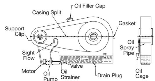
All chain drives should receive regular maintenance. Each drive should be inspected after the initial 100 hours of operation. Thereafter, most drives may be inspected at 500 hour intervals. However, drives subject to shock loads or severe operating conditions should be inspected at 200 hour intervals.
