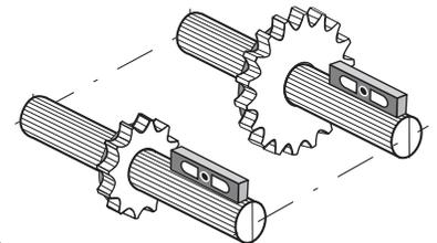
2. Sprocket axial alignment can be checked with a straight edge which will extend across the finished sides of the two sprockets. Normally, it is good practice to align the sprockets as close to the shaft bearing as possible. For long center distances, use a taut cord, or wire long enough to extend beyond each of the sprockets. The maximum allowable amount of axial misalignment is obtained from the following formula:
