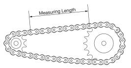
Measurement of Chain for Wear Elongation
