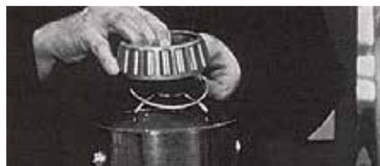
Hot oil pots, with a tray or hook to support the bearing cone (inner race), effectively ease the installation of tight inner races on shafts.
