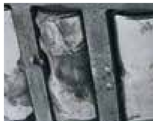
Full race width fatigue spalling: caused by heavy loads creating a thin lubricant film and elevated temperatures.
