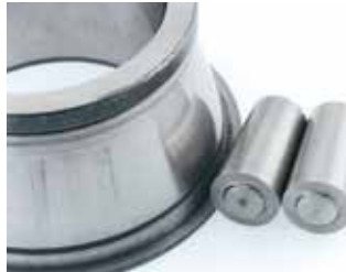
Abrasive wear: Fine abrasive particle contamination.
