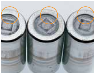
Roller end scoring: Metal-to-metal contact from breakdown of lubricant film.
