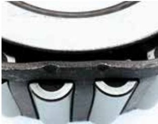
Cage deformation: Improperly installed or dropped bearing.
