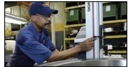
Duke Brown performs a final build up of a tapered bearing. This involves measuring the bearing in order to set the lateral clearance.
