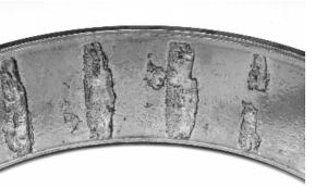
Figure 3: Etchingor corrosion.
