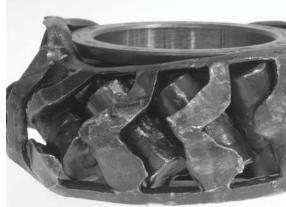
Figure 1: Total bearing lockup.
