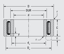
ADAPT bearings are interchangeable with ISO toroidal and spherical roller bearings.
