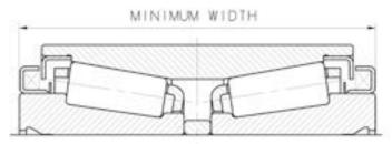
Minimum bearing assembly overall width after reconditioning or remanufacturing, from cone back face to cone back face (not including backing ring and axle end cap), must be within the following dimensions:
