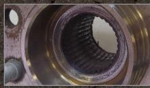
**Poor Performance:** Bearing cone can turn on the hub barrel, which changes the bearing setting – promoting vibration, excessive noise and premature wear.
