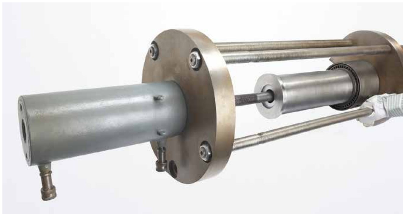
Fig. 29 Holding the pulling shoe down against the bearing face bearing puller
