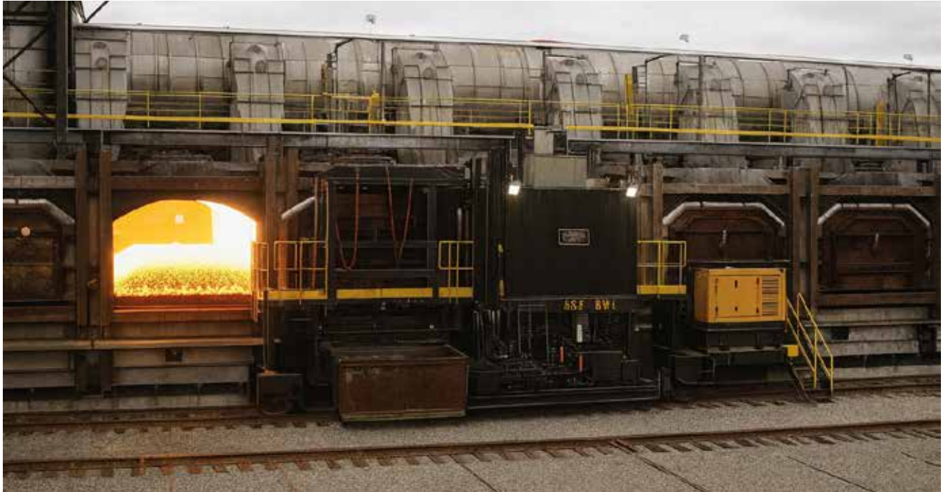
Fig. 20 Coke transfer car equipped with AP bearings
