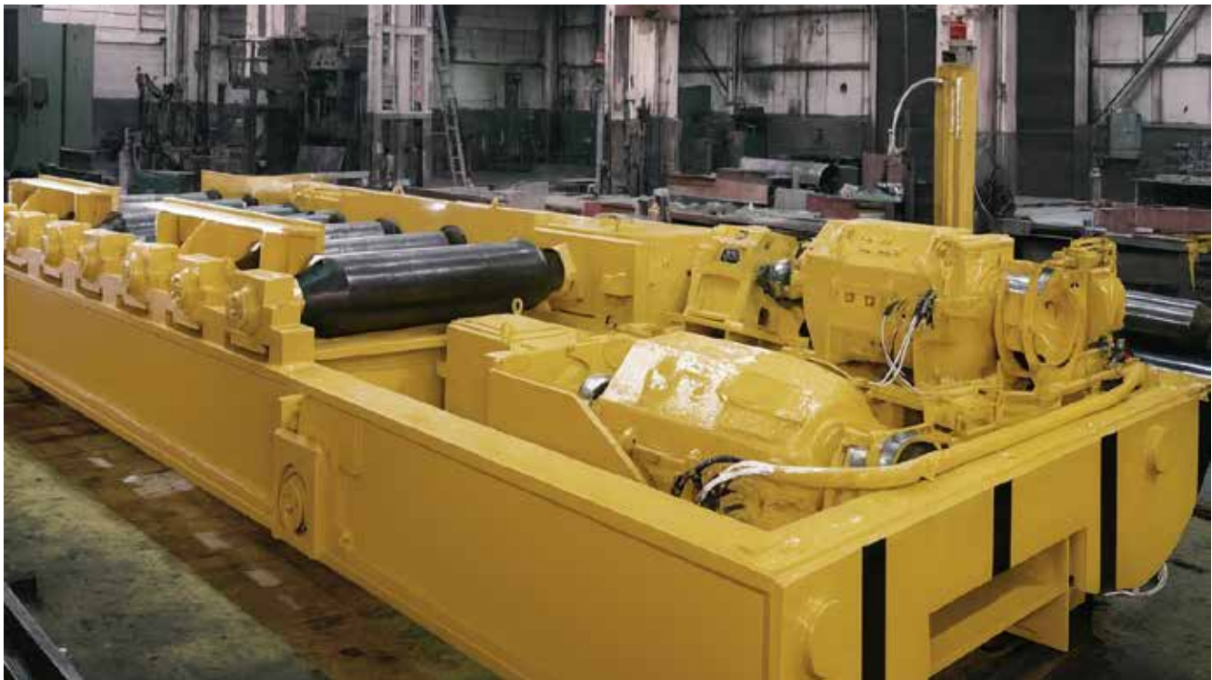
Fig. 10 A standard narrow adapter is used at both positions to ensure positive radial location of the AP bearing cups. A close clearance is provided between thrust lugs and the sides of the adapters to keep axial movement of the roll to a minimum.
