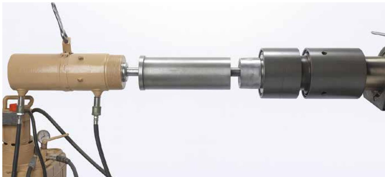
Fig. 28 Tooling used to push bearing onto shaft
