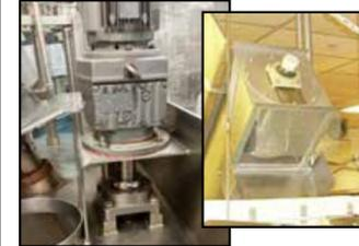
Type E Solution® bearings for large shafts (to 5" / 127mm), and Poly-Round® bearings for standard shafts (1/2" to 3" / 12.7mm to 76.2mm), are the most sanitary bearings available: no contamination, no corrosion, and no need to re-grease after washdown.
