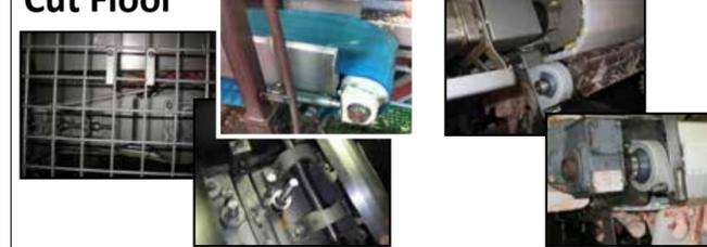
On tension devices (flat belts, overhung loads) and high speed saws (hock cutters and others), EDT mounted ball bearings with solid lubrication in non-corrosive housings elevate food safety and extend up-time.
