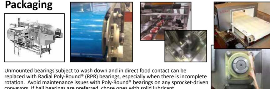
Unmounted bearings subject to wash down and in direct food contact can be replaced with Radial Poly-Round® (RPR) bearings, especially when there is incomplete rotation. Avoid maintenance issues with Poly-Round® bearings on any sprocket-driven conveyors. If ball bearings are preferred, choose ones with solid lubricant.
