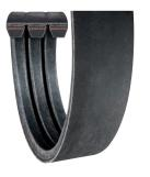
Banded version of Super Blue Ribbon belt. It's an ideal choice on classical v-belt drives where individual belts tend to rollover or whip severely due to fluctuating load conditions or harsh drive vibration. The individual ribs are permanently joined together at the top with a reinforced fabric tie-band. Super Vee-Band belts also provide oil and heat resistance and static dissipation.
