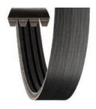
Specially designed and constructed to meet the unique demands of the forestry industry. It's designed to slip during "overload" or drive stall conditions. By allowing the belt to have controlled slippage, less heat is generated, which results in longer belt life.
