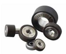
EDT Radial Poly-Round® bearings (RPR's) are manufactured from bearing grade polymers and 316 stainless components, and are designed to directly retrofit deep groove ball bearings and other styles of radial bearings.
