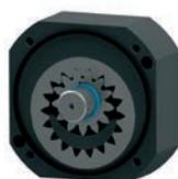
Internal gear pumps have two gear wheels, of which the outer (ring gear) is internally toothed. The sprocket running inside is smaller. The fluid is conveyed in the spaces between the tooth gaps of the two gear wheels.
