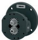
The external gear pump consists of two intermeshed gears. One of the two gears is driven by a shaft. The second gear wheel (idler gear) is pulled along via the toothing. When the wheels engage, the tooth gap is closed by the opposite tooth. Negative pressure occurs when a tooth emerges from the gap. This free space sucks in oil.
