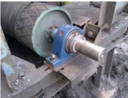
*Head Pulley with Spherical Roller Mounted
