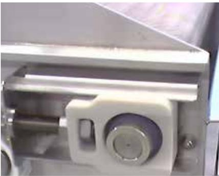
*Polymer Plain Bearing Used on Take-Up Position of Sprocket-Driven Conveyor*
