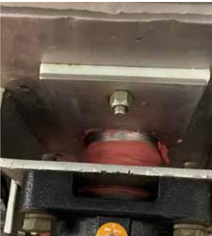
*Type-E Roller Mounted Bearing Unit with a Stand-Off Bracket on a Screw Auger*
