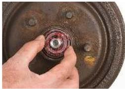
the rotor/hub assembly back over the spindle. After following Step 4, pack the outer bearing cone assembly with grease. Install the
