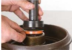
assembly in the hub, then install the new seal. Make sure the seal lips are pointed in the right direction following the vehicle manufacturer's specification. Use the proper seal installation tool.
