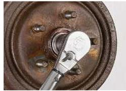
lbs. while turning the rotor. Back off the adjusting nut 1 full turn. Re-torque the nut to 10 ft. lbs. while turning the rotor. Next, back off the adjusting nut 1/4 turn. Lock the nut with a new cotter pin.
