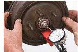
Push the rotor in while oscillating and read the dial indicator. Pull the rotor out while oscillating and read the dial indicator again. The bearing end-play is equal to the total indicator movement, which should be between 0.001 in. and 0.005 in. If not, repeat steps 7 and 8. Reinstall all components as the vehicle manufacturer recommends.
