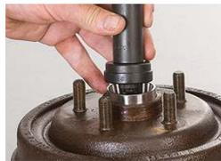
cup and outer cup into the hub/rotor assembly until solidly seated against the hub shoulders. Be careful not to damage the cup surfaces. Never use a bearing cone assembly to drive a cup.
