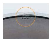
**Bearing cup (outer race) -face denting:** Indentations from hardened driver.
