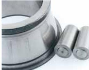
**Abrasive wear:** Fine abrasive particle contamination.
