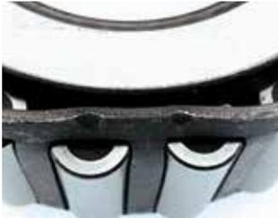
**Cage deformation:** Improperly installed or dropped bearing.
