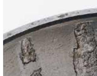
**Line spalling:** Roller spaced spalling from bearings operating after etching damage.
