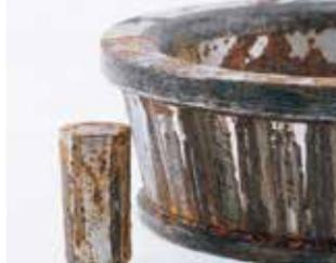
**Etching:** Rusting with pitting and corrosion from moisture.
