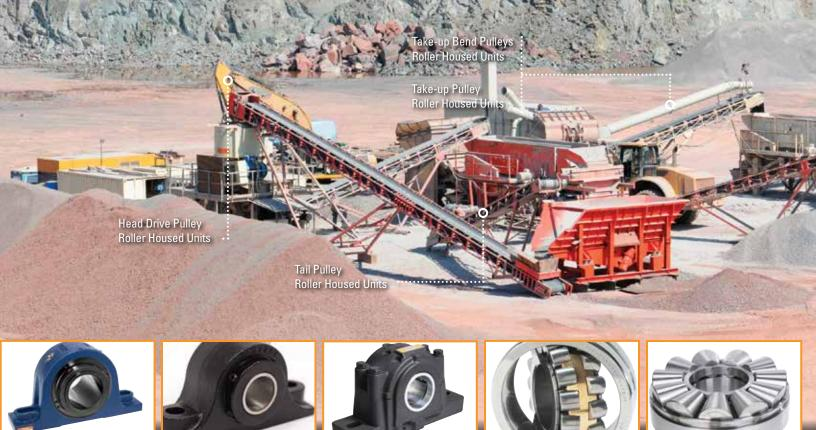
Spherical Roller Bearing Housed Unit
