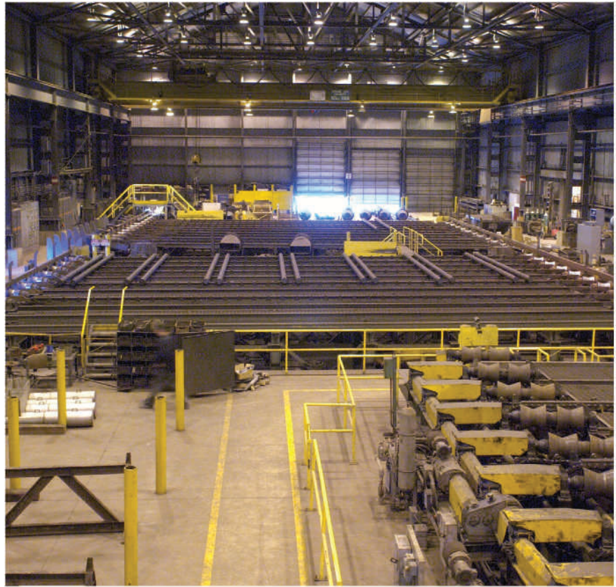
Cooling Table at Continuous Thermal Treatment Facility
