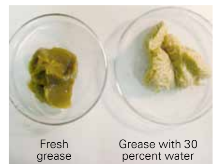
Fig. 1 - Effect of water on grease.
