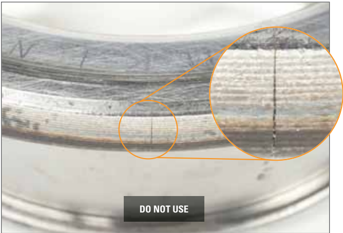
Fig. 14. Cone large rib cracks.
