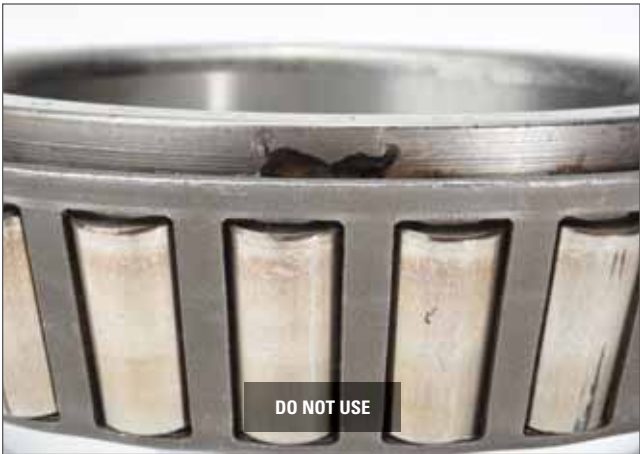
Fig. 16. Example of fractured large rib.
